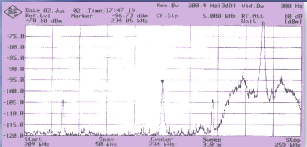
**Fig. 4: The 234kHz signal and its sidebands reduced by 26dB whilst hardly affecting the 252kHz station.**
