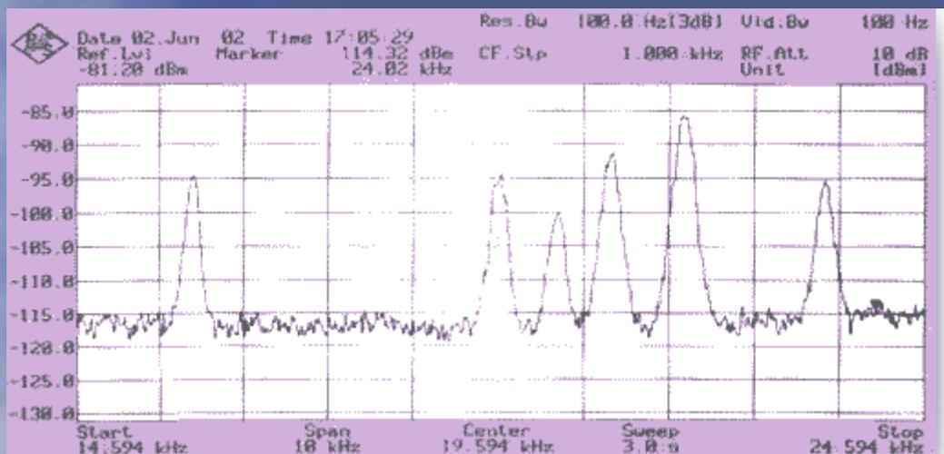
**Fig. 5: The spectrum of signals centred on 19.6kHz with the one on 24kHz nulled.**
