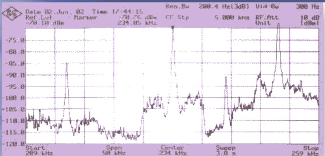
**Fig. 3: The display centred on a signal at 234kHz signal pre-nulling.**
