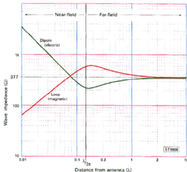
**Fig.1: Wave impedance, high for E-Field and low for the H-field. The commonly accepted impedance plots for the near to far field transition.**
