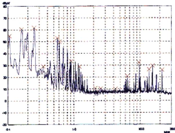
**Fig.3: The Rohde & Schwarz screened loop 150kHz to 30MHz**
