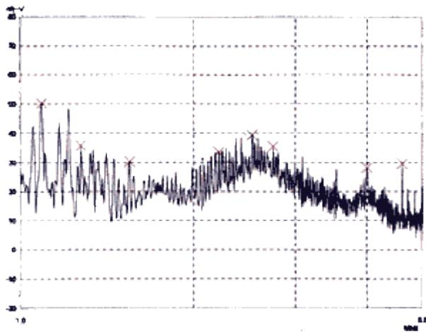
**Fig.5: The off air signals from the Rohde & Schwarz active whip**
