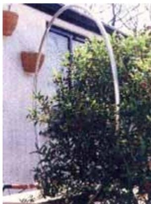
indoor use does yield results, even in my computer infested home, with all the resultant radiated hash, don't consider it as a solution. Once I located the ALA 1530 outside of the electrical field of the house, generated by all that mains wiring, then the antenna really came into its own, but then you'd expect that, wouldn't you?
